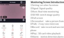
②Signal: Signal quality 3Horn: Real-time monitoring @SD/HD: switch image quality ⑤Full screen (1)Screenshot: take a picture from the video (2)Talk: 2 way voice intercom (3)Record: take record and save into the mobile (4)Play: SD card video playback
