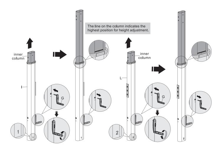
Attach the handle to the column marked with "1". Attach the handle to the column marked with "2".
