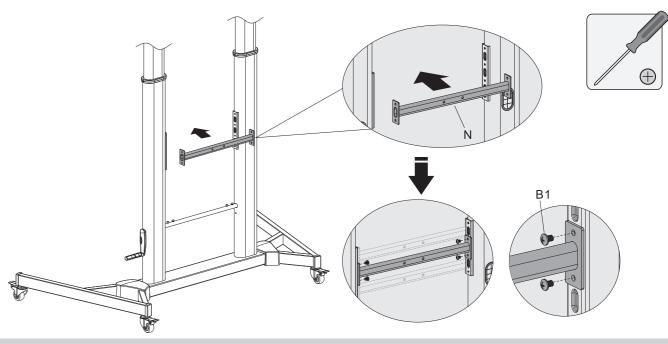
Install the support bar to the columns at the desired position and secure using the appropriate screws.
