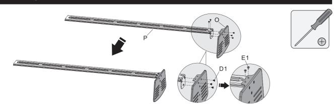
Attach the camera shelf to the connecting plate with the appropriate screws. Tighten all screws using a proper Phillips screwdriver.
