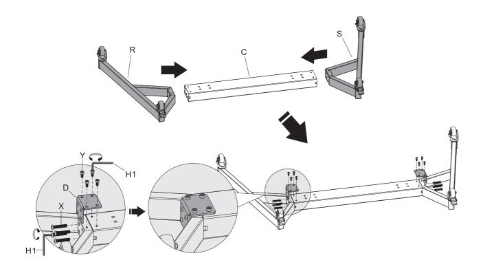
Insert the right leg into the base. Align the holes on the right leg to the holes on the base. Fix the base with the connecting pieces and the screws. Repeat this step for the left leg.
